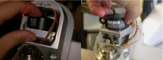
6. Gently place the motor/encoder to the side of the kappa axis. You can now spin the interlocking gear that the motor attaches to and verify that it moves freely and is in working condition.
