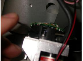
9. Insert the encoder brace to secure the encoder wheel before loosening the second screw.
