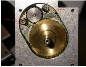
14. Remove the two allen-head screws that attach the motor to the encoder assembly.
