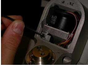
5. Grasp the assembly and "roll" it out of position taking care to watch the wires.
