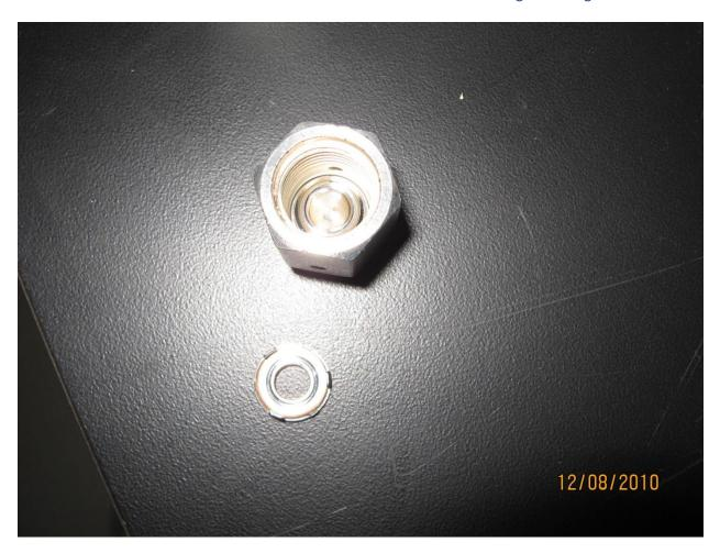
9. Attach Fitting: Shows the fitting attached to the detector. Turn on the pump and vacuum for 15 minutes.
