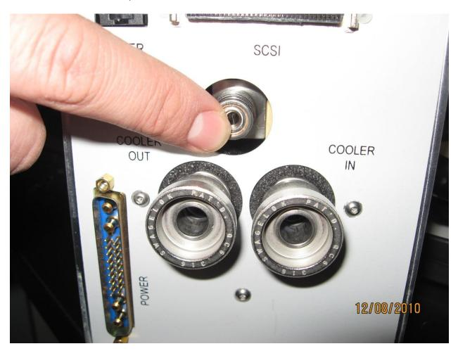
8. Detector Nut + Insert: The insert inside the nut is needed when attaching the fitting.
