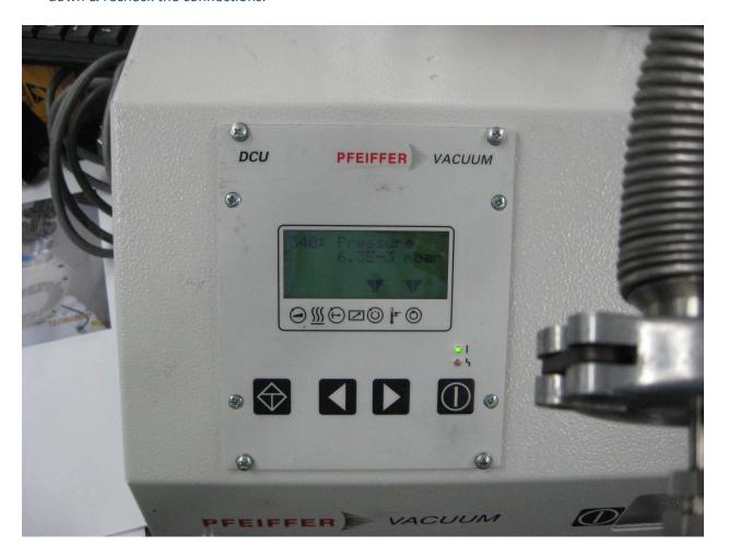
Allow the detector to be vacuumed a minimum of 4 hours (overnight is fine).
