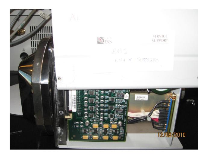
6. Apex II Cover removed: This is what the detector looks like when you remove cover.
