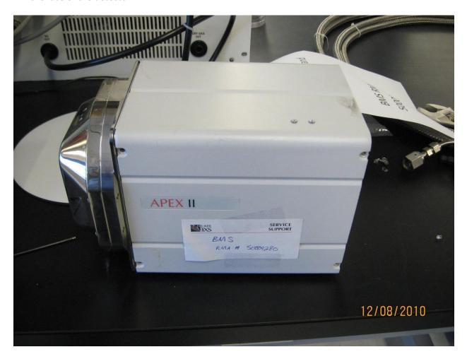
4. Apex II Cover: The cover needs to be lifted up to remove it. Do not slide it back.
