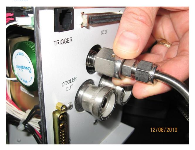
10. Valve: After vacuuming for 15 minutes, the valve on the side needs to be opened. The vacuum needs to reach  $^{\sim}5$  x 10-5 before opening. If this value is not reached in 15 minutes then shut down & recheck the connections.
