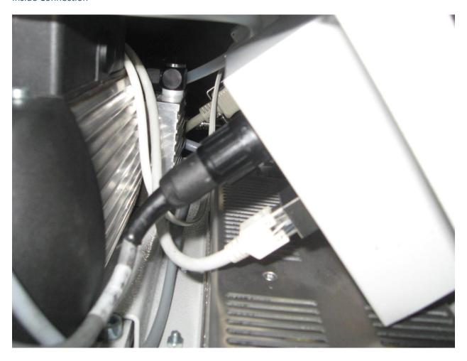
3. Apex - 4 screws need to be removed to take the cover off. 2 on each side (top & bottom) near the face of the detector.
